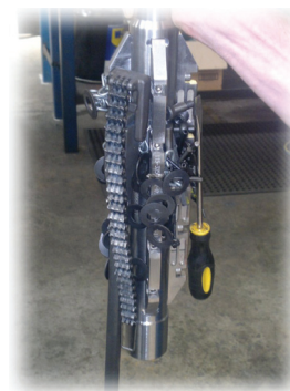
Surface demonstration of magnet strength
